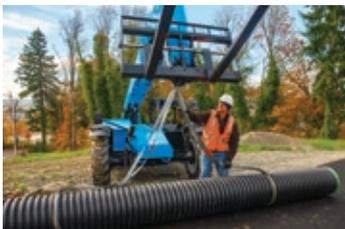
All Genie telehandlers come equipped with a lift shackle that enable you to sling a load without secondary attachments. A factory lift shackle lift chart provides clear capacity limitations to the operator.
