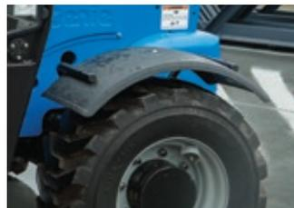
Fenders are also standard keeping the machine cleaner as well as shields the operator from mud being slung.
