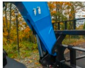
Auxiliary hydraulics ensure all Genie machines can be equipped with attachments requiring hydraulic connections.
