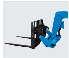
Three simple quick-attach interfaces ensure that you can leverage attachment investment between machines.\*
